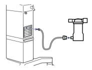
Disconnect the Servo Ultra Nebulizer from the ventilator.
