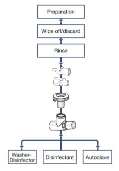
Only the Aerogen Pro Nebulizer unit, T-piece and neonate adapters can be autoclaved.
