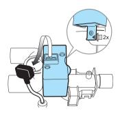
Disconnect the O<sub>2</sub> sensor and carefully unlock the latches.
