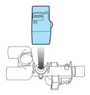
Put the O<sub>2</sub> sensor in position.
