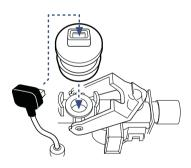
Connect the O<sub>2</sub> cell connector and put the O<sub>2</sub> cell in position.
