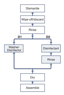
There are two disinfection procedures for the expiratory cassette and associated parts, D1 and D2. In D1 (recommended) a Washer-Disinfector (EN-ISO-15883-1) is used, and in D2 a disinfectant is used.
