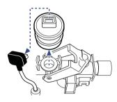
Disconnect the O<sub>2</sub> cell connector and lift out the O<sub>2</sub> cell.
