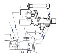
Put a new bacterial filter in position and connect the filter to the tube.
