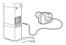
Disconnect the Capnostat sensor and airway adapter from the ventilator.
