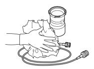
Wipe the nebulizing chamber and control cable with a soft cloth moistened in soap & water or detergent-based disinfectant.
