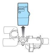
Lift the O<sub>2</sub> sensor out of position.
