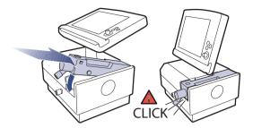
Hinge the expiratory cassette and press it firmly down into lock position.
