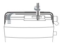
Turn the bayonet screw one quarter of a turn to release.
