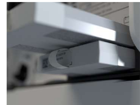
Two hot-swappable batteries with a total of three hours of run time.
